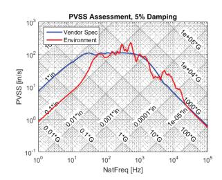
Using Kornucopia's k\_SRS function it is easy to compute shock response spectra results on transient acceleration data coming from physical tests or transient simulations. The PVSS result above, presented on a Kornucopia 4CP plot, indicates the spec is exceeded.
