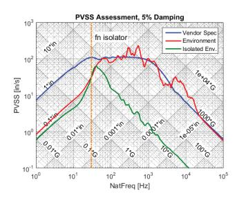
The final SRS assessments presented using both the Absolute Acceleration form and the Pseudo-Velocity form. Each of these plots is produced using only the  $k\_SRS$  function to compute the results and the  $k\_plot$  function to create the automatically labeled plots. Kornucopia's Units Engine makes it easy to calculate and plot in a variety of other units as needed.
