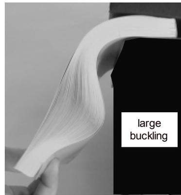
**Figure 2. Deformation characteristics of a soft-cover book.**
