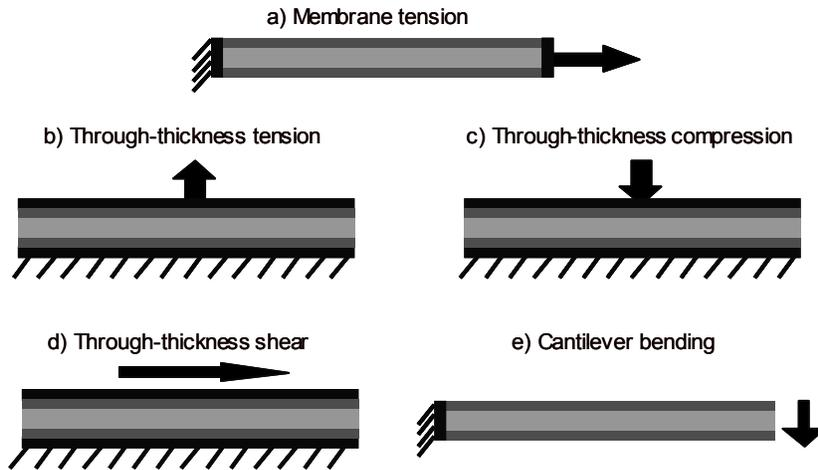
Figure 4. Global deformation modes utilized to calibrate model.
