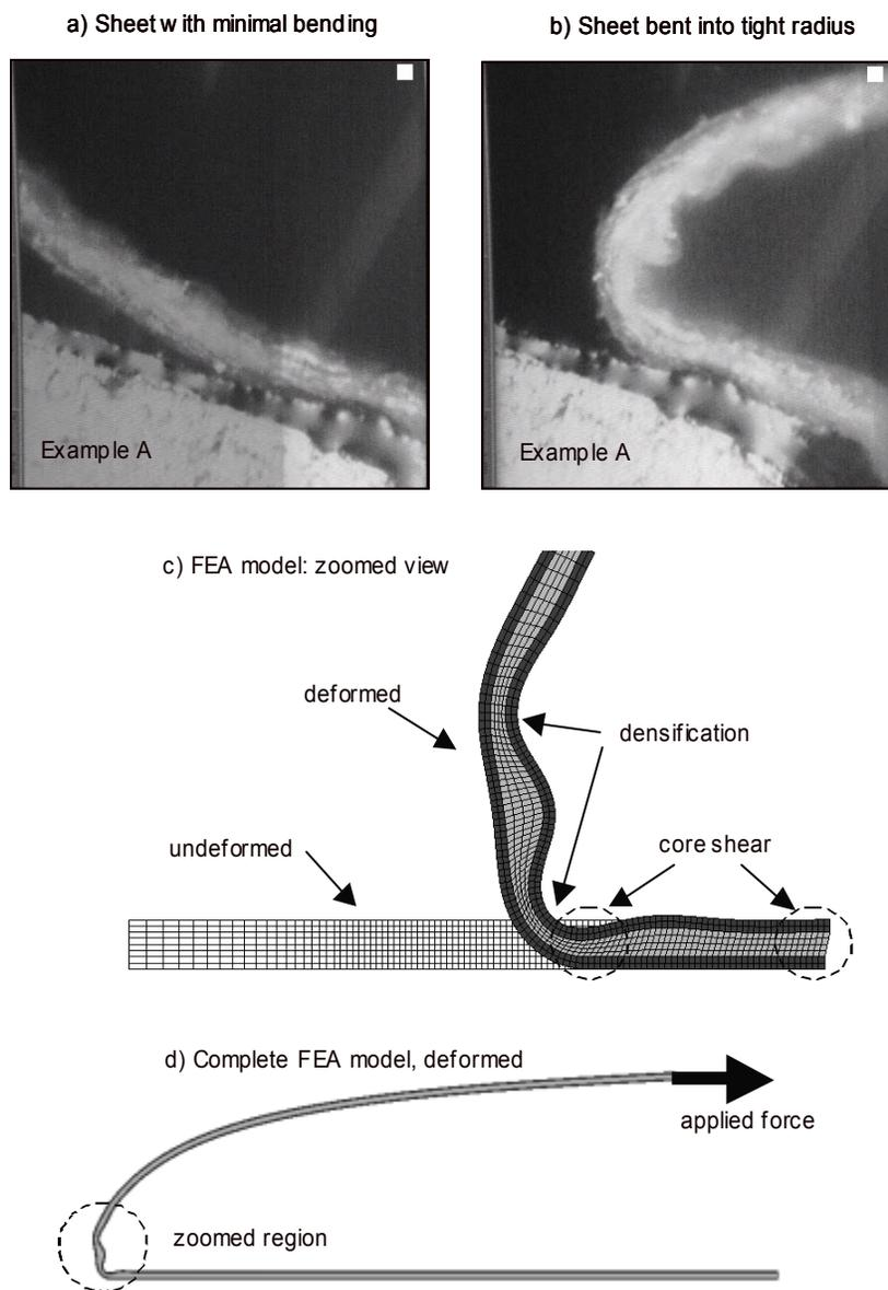
Figure 7. ABAQUS/Standard model's response to a tight bend.
