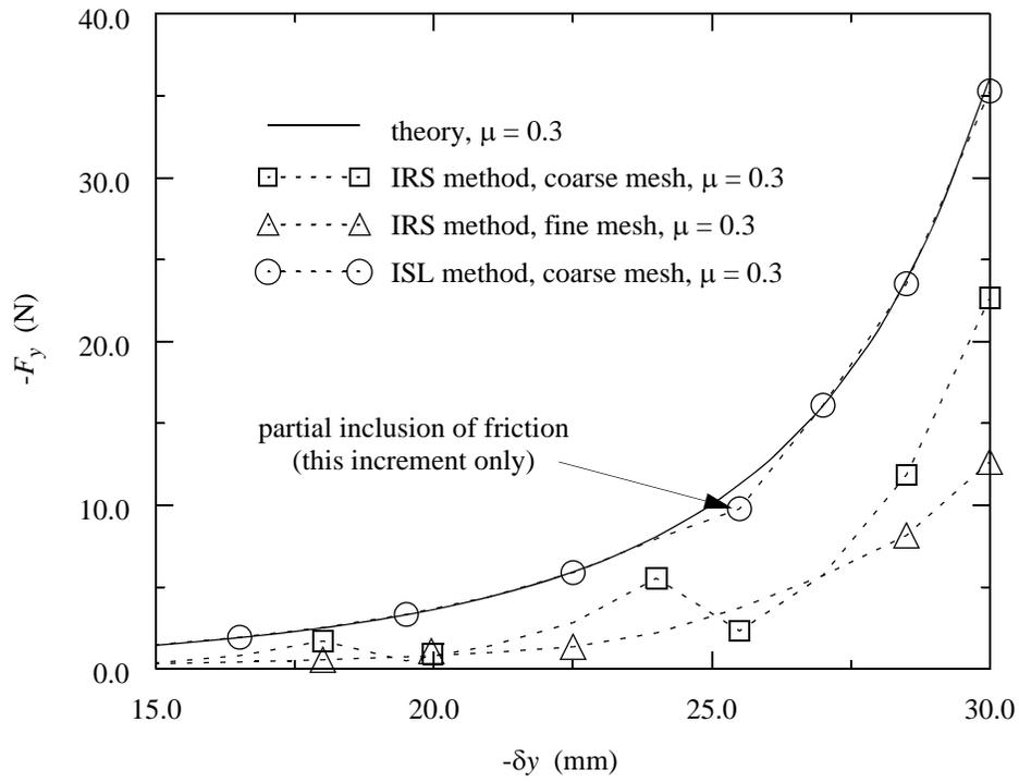
**b) FE Results using *modified* friction implementation**
