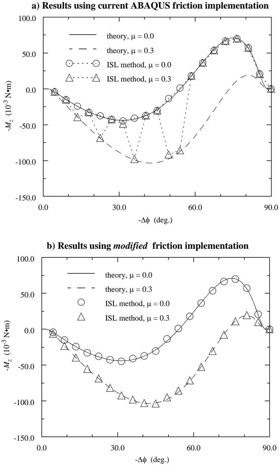
**Figure 8: Further demonstration of solution accuracy with modified friction implementation: second example problem.**
