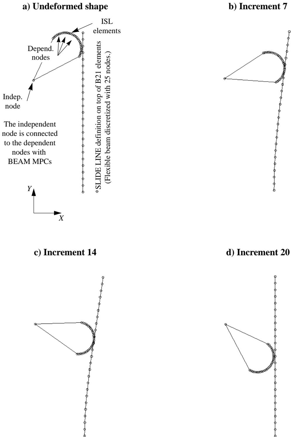
**Figure 7: ISL Model of second example problem: simulation of a rigid cam being rotated into a flexible member.**
