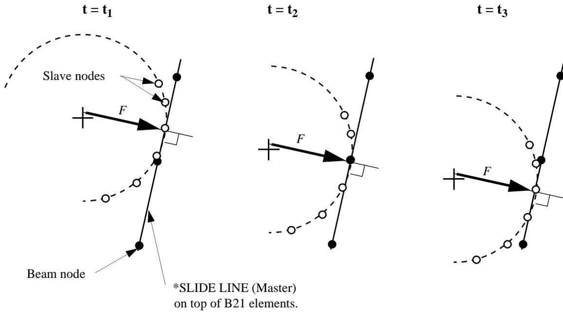
Note: In a Master/Slave contact algorithm, the slave node is not allowed to penetrate the Master surface. Nothing prevents the Master surface from penetrating the surface between the slave nodes.
