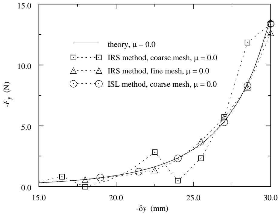
**Figure 4: Comparing different FE models of first example problem without friction.**
