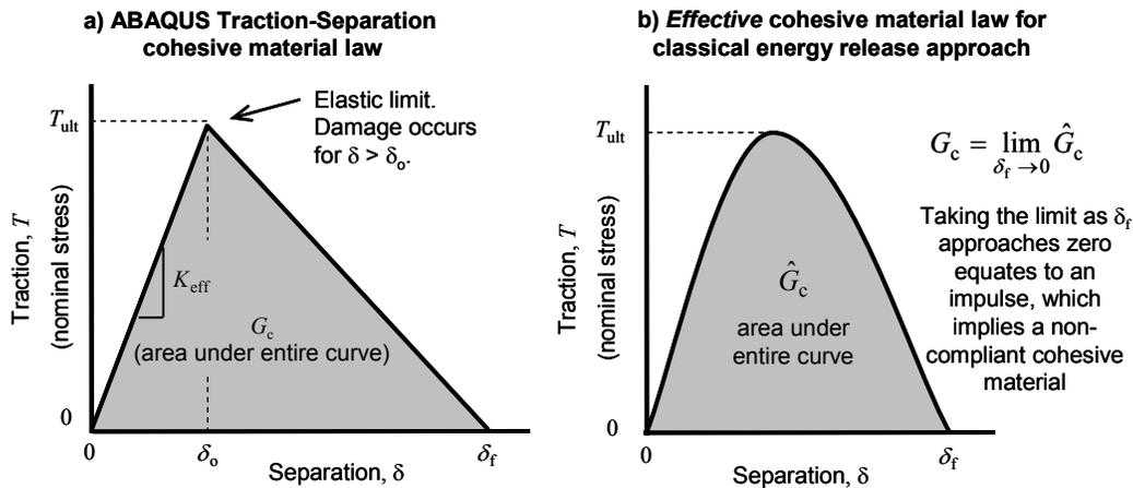
**Figure 5. Traction-separation law utilized in finite element cohesive model and an interpretation of the classical Griffith energy release approach cast in a cohesive material law form.**
