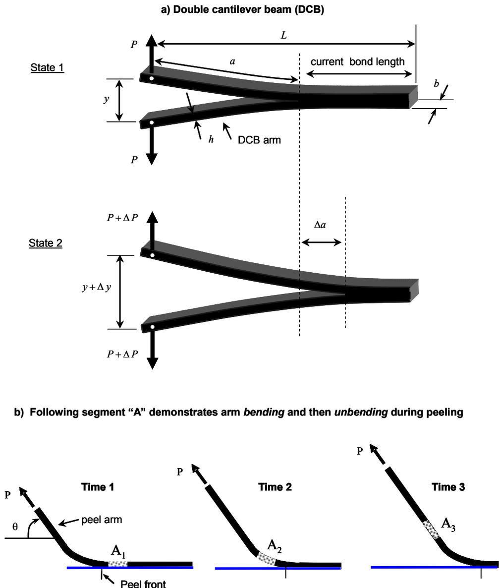
Figure 1. Idealized crack growth in a DCB specimen and the deformation history during single arm peeling.
