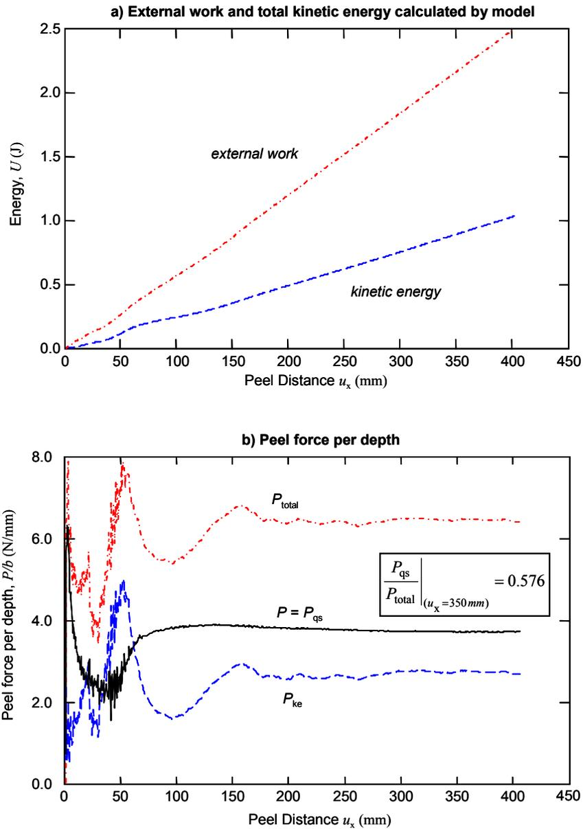
**Figure 6. Improving calculation of peel load by compensating for excessive kinetic energy in Explicit model. Results shown for modeling approach #1 (solid aluminum mesh and solid epoxy mesh), Case 7 ( $\delta_f / \Delta L_{\text{COH2D4}} = 1.0$ ), and  $G_c = 1.32 \text{ kJ/m}^2$ .**
