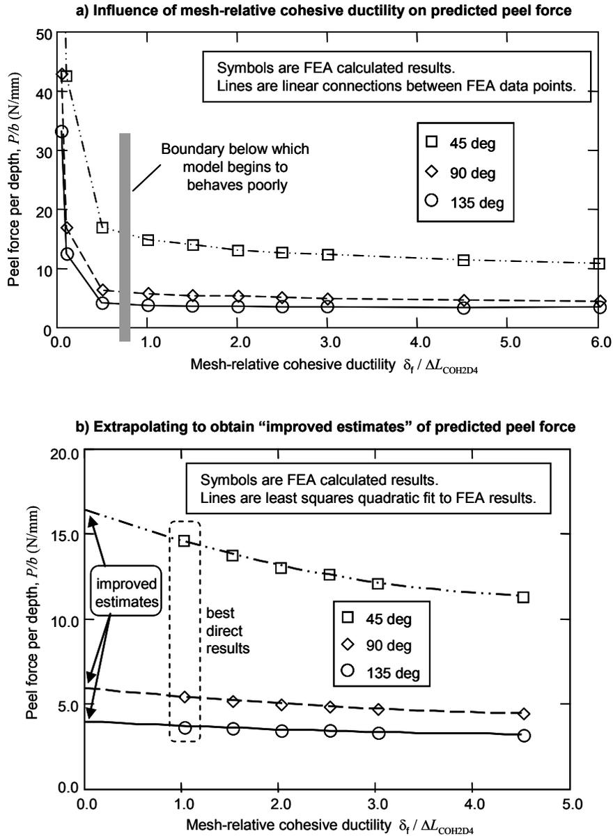
**Figure 7. Influence of mesh-relative cohesive ductility on FEA predicted peel force and an extrapolation method to obtain "improved estimates." Results are for modeling approach # 1 with  $G_c = 1.32 \text{ kJ/m}^2$ .**
