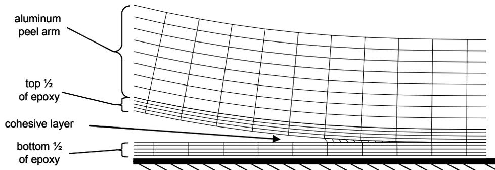
Figure 4. Various finite element modeling approaches utilized in peeling study.
