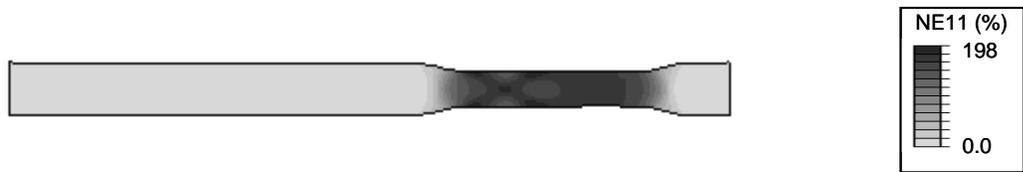
**c) Local nominal strain measure NE11 at an apparent nominal strain of 34 %**
