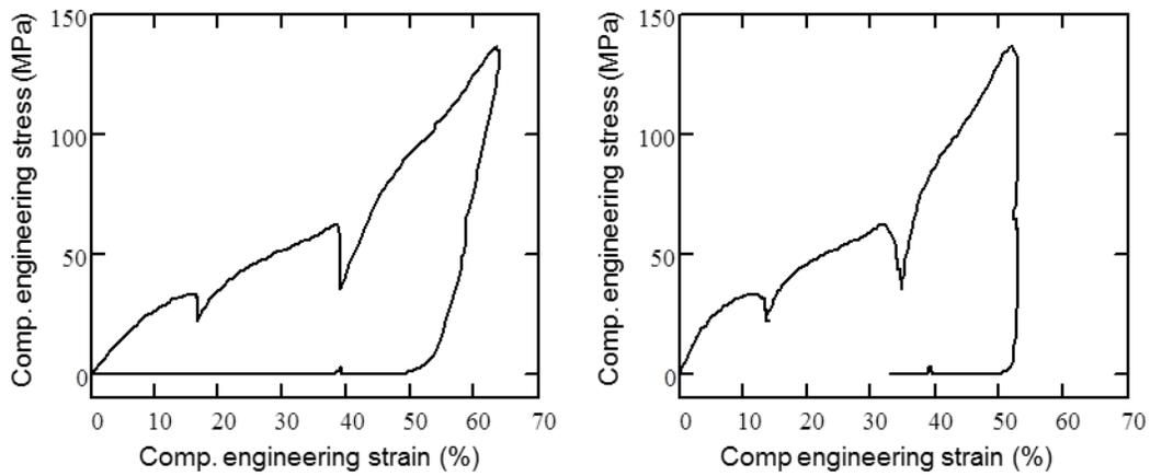
a) Strain computed from cross-head displacement
