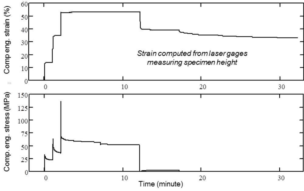
c) Strain and stress data as a function of time
