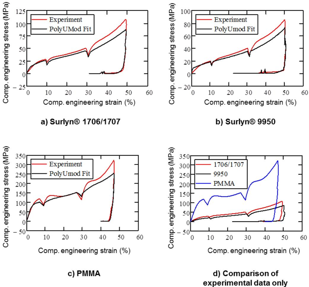
**Figure 6: Summary of material test data for three polymers studied and their PolyUMod® fits. This figure shows only evaluation of a low strain rate of  $0.005 \text{ s}^{-1}$ . The PolyUMod® calibration actually used both the low strain rate data (shown) and high strain rate data (not shown for brevity) in the nonlinear calibration procedure.**
