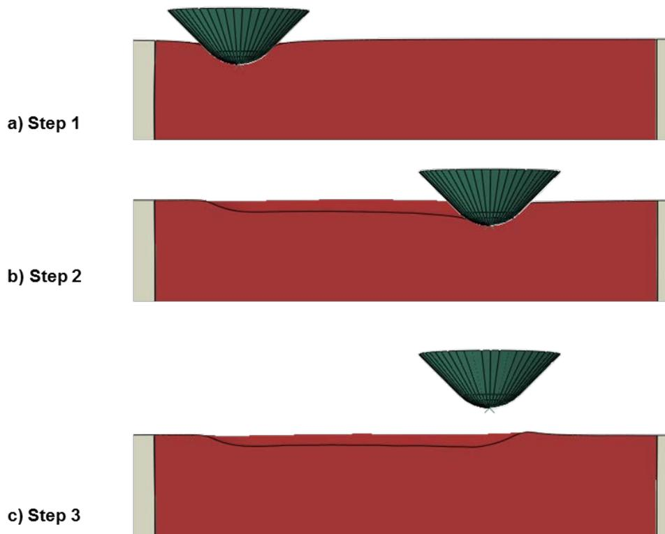
**Figure 8: The scratch simulations were performed in 3 steps: (1) Push the indenter down into the material, (2) scratch the surface by moving the indenter horizontally, (3) unload the indenter and let the material relax.**
