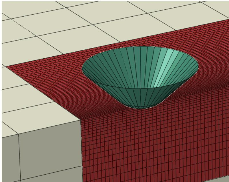
**Figure 7: Finite element mesh used to represent a 100 micron tip indenter scratching a polymer surface. The model is using half symmetry.**
