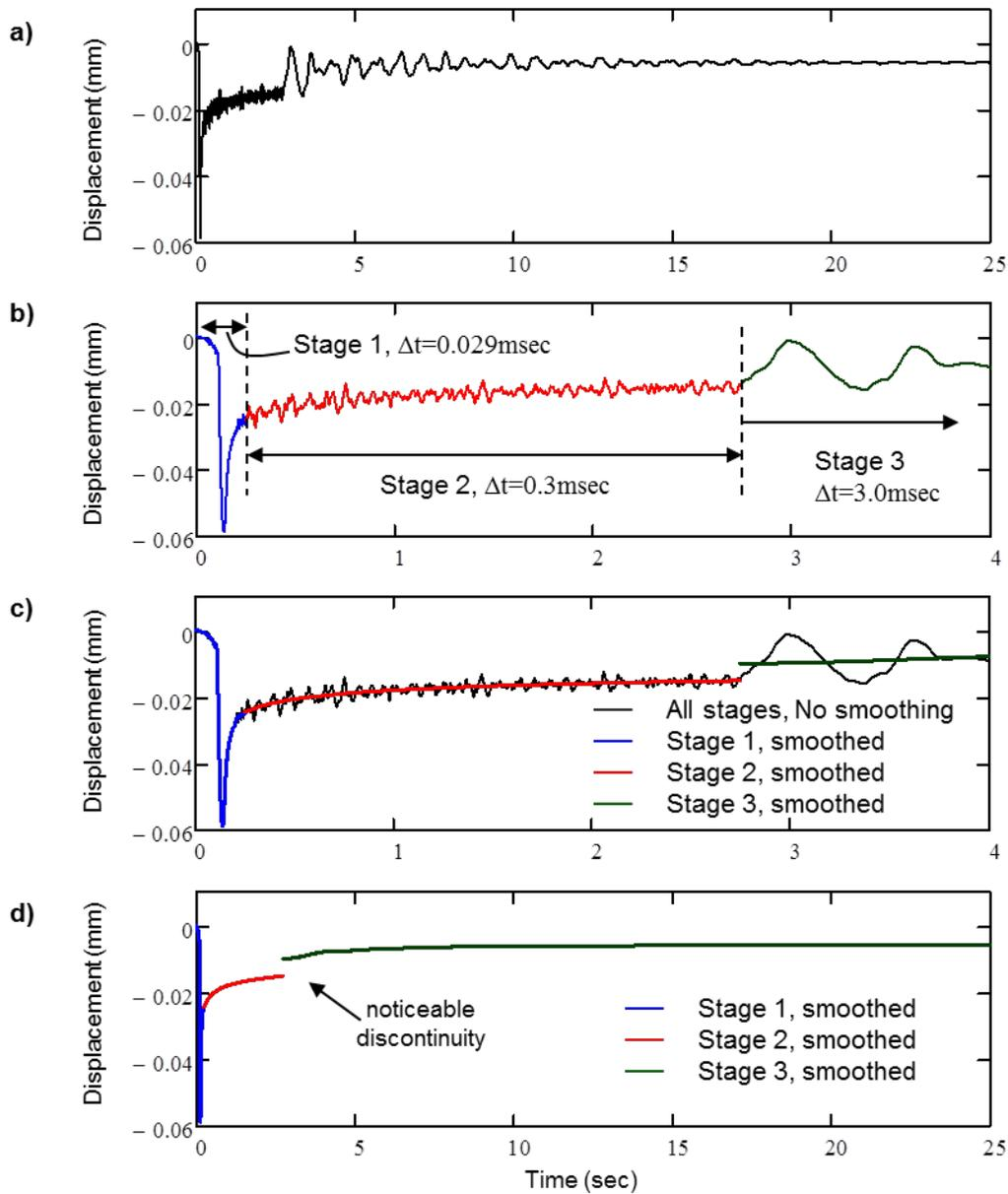
**Figure 9: Assessment of the influence of using three different stages of mass scaling to speed up solution. Data shown is for a scratch simulation of Surlyn® 1706/1707. The data shows the creep recovery of a single node on the polymer’s surface along the scratch path.**
