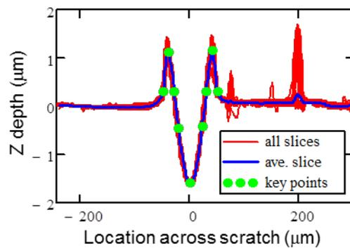
c) Healed PMMA data (1,000mN scratch load) with additional Kornucopia® processing
