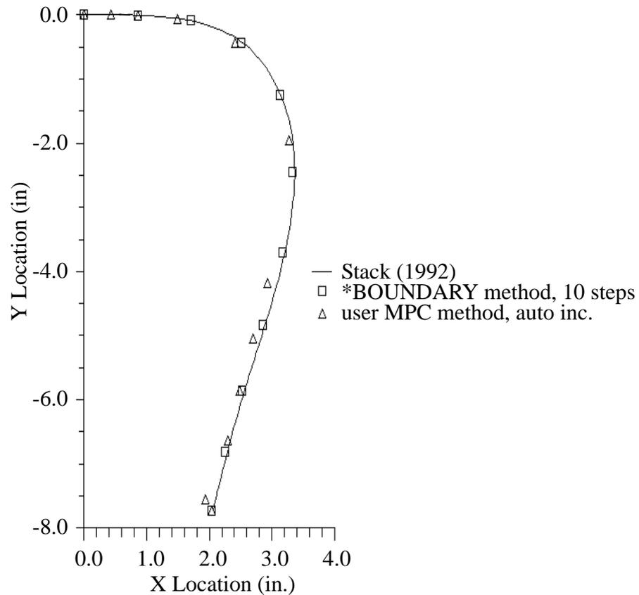
FIGURE 4. Quasi-static feeding of a thin sheet into a gravity field.
