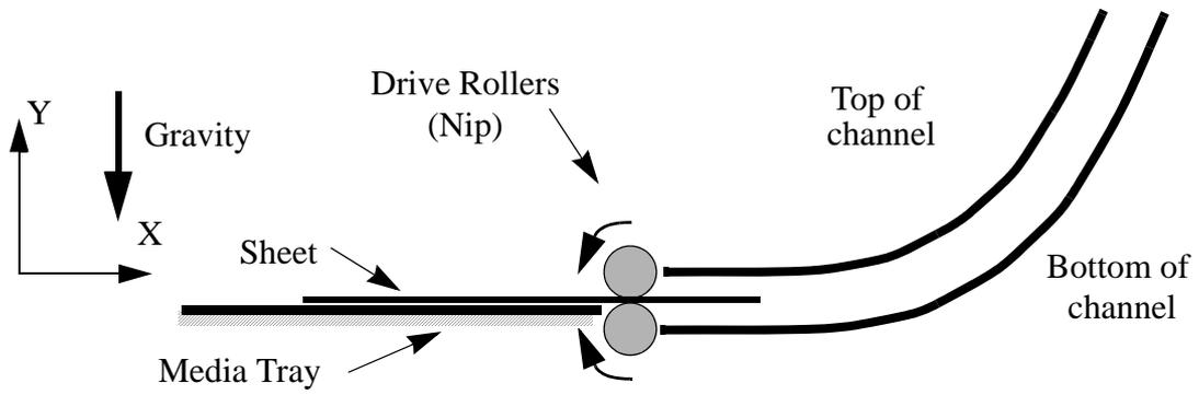
**FIGURE 1. Schematic of sheet being transported into a channel.**
