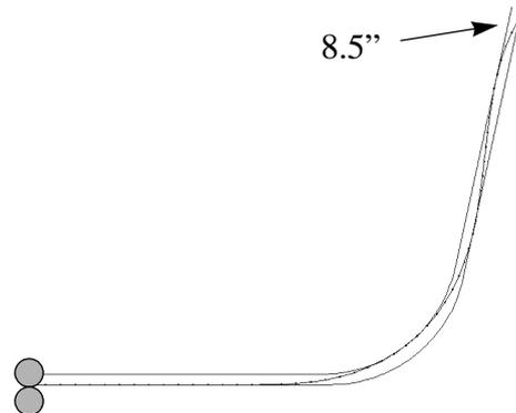
**FIGURE 6. Feeding straight and curled media into both open and closed channels: Deflected shapes for different feed distances. Gravity loading is included.**
