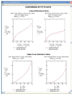
Mathcad was used to document and study fundamental issues with hyperelastic material models. The document compares closed-form analytical results to experimental results. Experimental results (below) were used to develop an understanding of how to use this hyperelastic approach inside Abaqus FEA.
