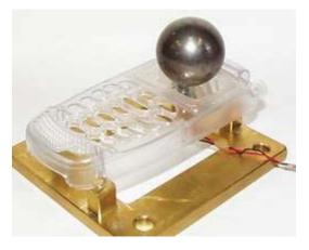
While working on the iDEN line of cell phones at Motorola, the author dropped a steel ball 0.5 m onto the phone cover, collected data, and then simulated the event in FEA software. Combining applied mathematics software such as Mathcad, and nonlinear FEA software such as Abaqus, lets users incorporate nonlinear closed-form analysis, real-world FEA simulations, and complex experimentally measured material behavior into a cohesive engineering analysis.
