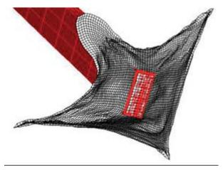
Products made of Kevlar, such as military and police vests, can already stop high-speed projectiles. Mathcad and FEA programs can provide a way to model and test improved designs of the material that will have a good correlation to real-world performance.
